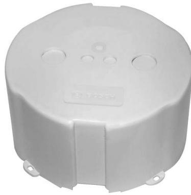
The back box is made from ABS material and is color matched with the ceiling loudspeakers. The Back box has knockout holes and is supplied with the cable glands. The unit can only be used as a back cover for LBD0606/10 and LCZ-UM12-IN ceiling loudspeakers. The back cover can be fitted to the ceiling loudspeaker frame by using the self tapping screws.
